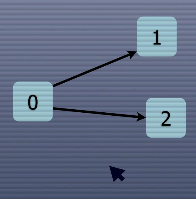
A representation of state 1 is sent to state space engine, which calculates and returns the successors
